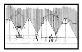
Figure n Multiple lights provide for consistent levels of lighting
