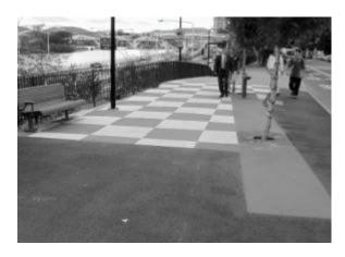
Figure h The use of different footpath patterns and colours is used in this example to highlight change of environment for cyclists and pedestrians.
