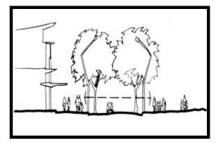
Figure d Landscaping is designed to minimise interference with sightlines
