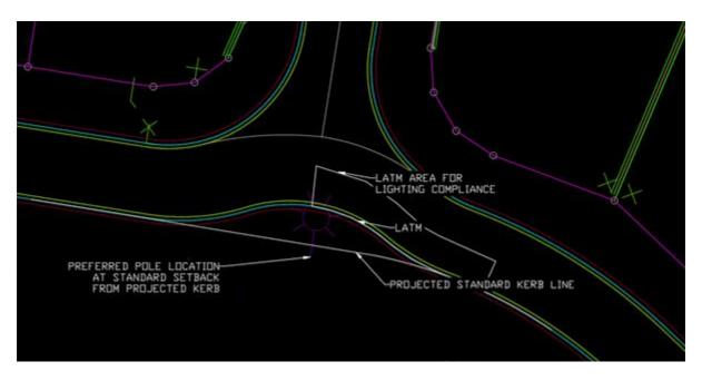
• If the area is not classified as an LATM device, it is preferred that a luminaire is installed at the location indicated and located at the standard setback from the projected kerb line.
