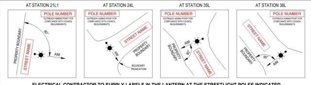
ELECTRICAL CONTRACTOR TO SUPPLY LABELS IN THE LANTERN AT THE STREETLIGHT POLES INDICATED Labels to be made for GROVOPLY II (1.5mm) or similar. Labels to be nominally 100mm x 100mm with black detail on white background
