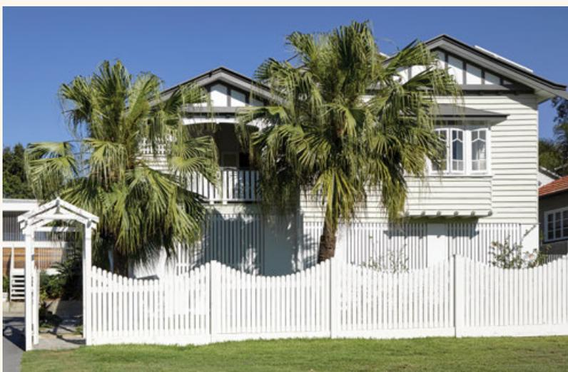
An example of a front fence that is low and does not block views to the house. The batted style of the fence allows gaps for openness and relates to the traditional style of the house and street. Privacy is achieved by layering the fence, vegetation and the verandah screening elements. The openness of the batten spacings allows views through to the hedge and garden beyond.
