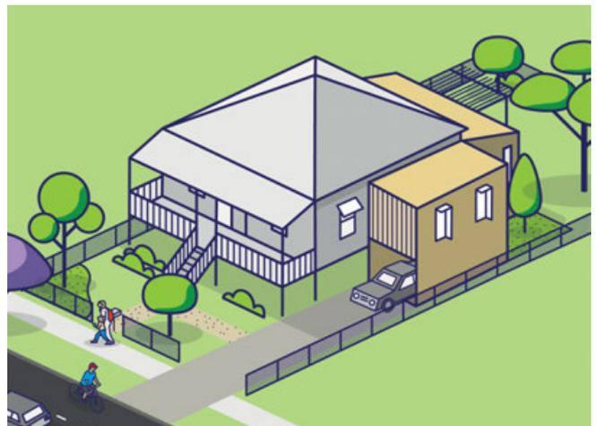
Locating an extension to the side and rear, setting new building work back from the front wall of the original house.
