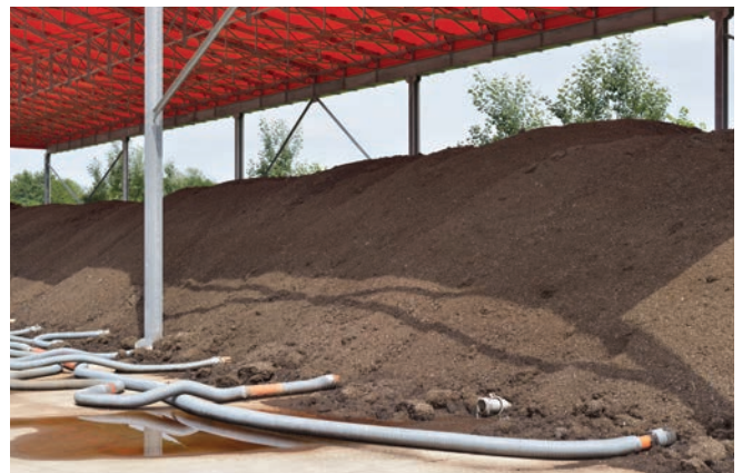
Picture: Active aerated static pile
